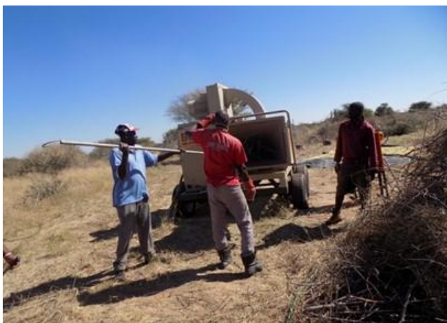
Feeding bush branches into machine. Only fresh part of woody leaves and pods feed into machine, all dead materials are removed to avoid mixing with fresh.
